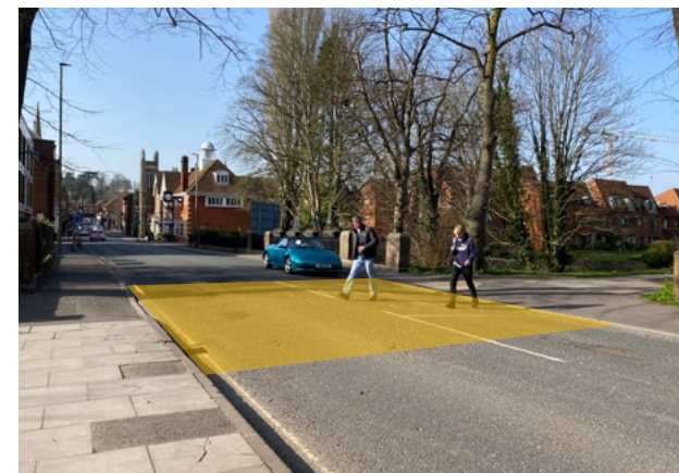
Figure 48. Indicative location (highlighted in orange) for a raised table to facilitate pedestrian crossings between Borelli Walk and Gostrey Meadow, and connections for people cycling between Borelli walk and proposed cycle facilities to/from Station Hill (proposal #4)
