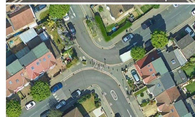
Figure 40. Example of a modal filter along a cycle route in Waltham Forest to reduce vehicle through traffic by requiring motor vehicle traffic to turn on approach to the junction. (see proposals 2 & 3) [source: Google Streetview (top, middle), Google aerial imagery (bottom)]
